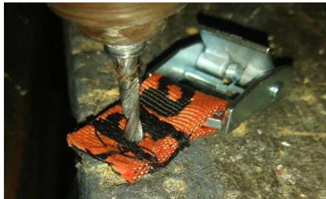
Figure 11: Drilling the hole into the buckle
