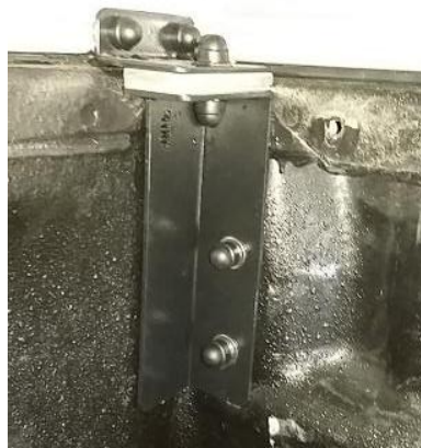
Figure 20: Mounting Universal-Front Support Bracket
