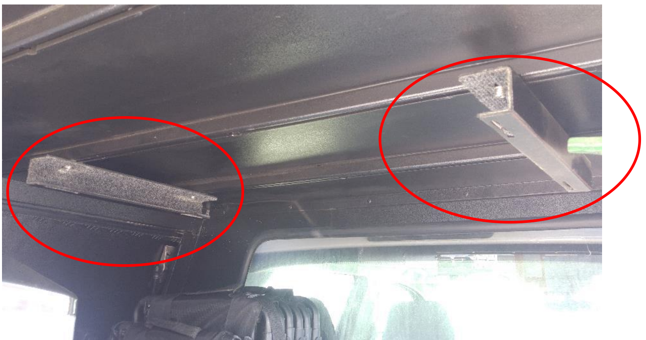
Figure 3: Table brackets installed
