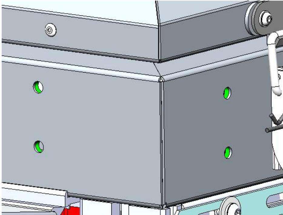
Apply unbroken beads of sealant around all of the laser cut holes, as well as making an unbroken bead around the perimeter, within the bounds of where the corner bracket will mount (AWN-CPR-000-006). See the image below:
