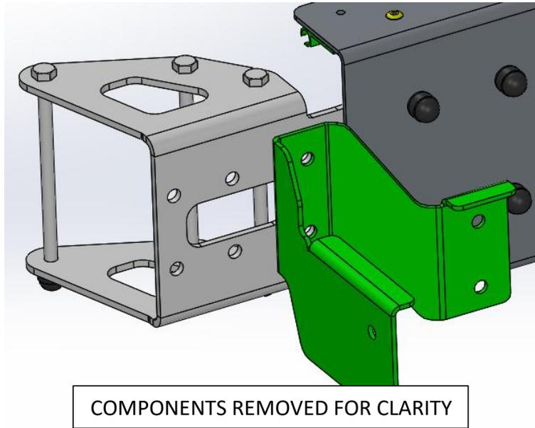
Align the front of the Shadow Awning, with the installed front bracket, as shown below. Insert the fasteners, as per the section *Component Identification*. Ensure that the awning is seated correctly, and not leaning forwards or backwards. Tighten these fasteners, and then tighten the fasteners on the rear corner bracket.
