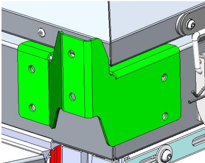
When inserting the fasteners, in the stack up order indicated under the section *Component Identification*, ensure that the two (2) plates, Awn-CPR-000-003, are aligned on the inside surface, as shown in the image below:
