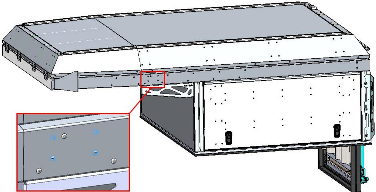
Apply unbroken beads of sealant around all of the laser cut holes, as well as making an unbroken bead around the perimeter, within the bounds of where the bracket will mount (AWN-CPR-000-007). Use the same technique, as described in *Fitment of Rear Mounting Bracket*.
