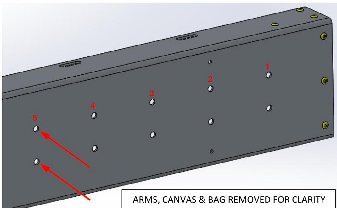
At the rear of the Shadow Awning, at the pivot point plate, count the hole pairs from the rear, and drill through the bag at hole pair three (3), as shown in the image below. Ensure that the arms, and/or canvas is safely out of the way before drilling. Use an  $\Phi 8.5$  mm drill bit.
