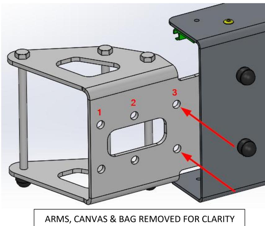
Align the rear of the Shadow Awning, with the installed rear corner bracket, as shown below. Insert the fasteners, as per the section *Component Identification*, do not fully tighten the fasteners.
