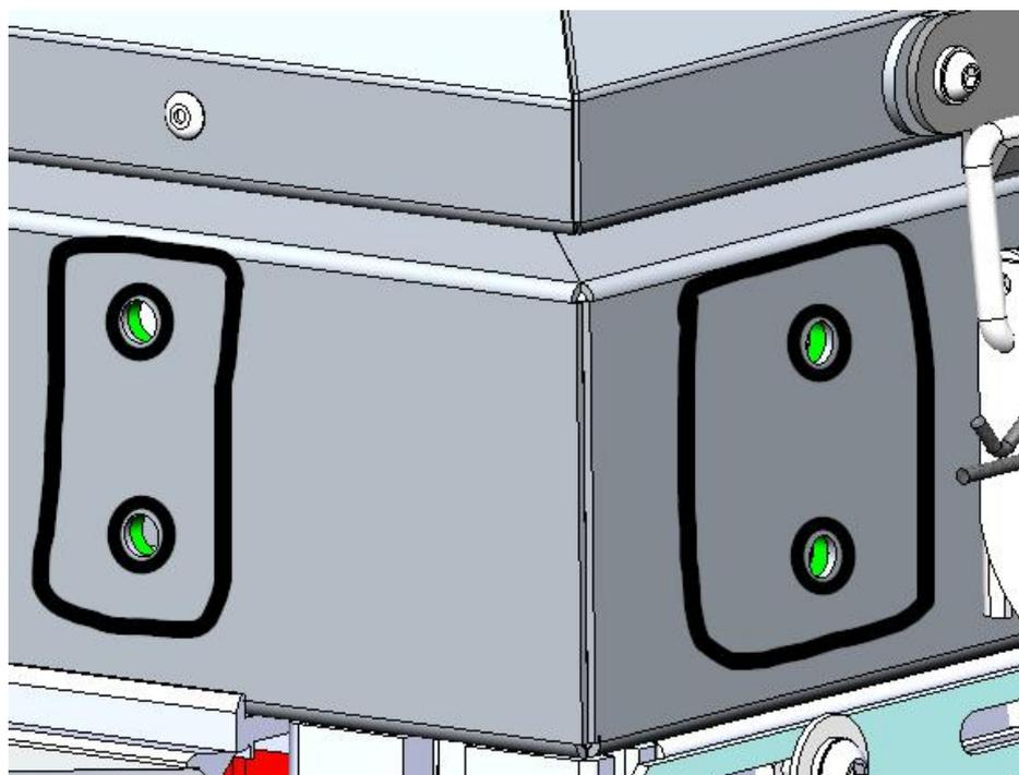
Align Awn-CPR-000-006 with the laser cut holes at the rear left hand corner of the Canopy Camper or Khaya, as shown in the image below:
