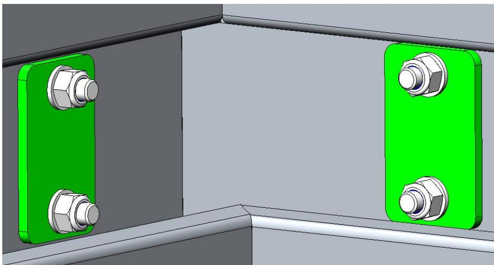
After tightening up the fasteners, wipe away any excess sealant that has squeezed out past the brackets, on the outside surfaces. The preferred cleaning agent is a 50-50 mixture of isopropyl alcohol and water. Refrain from using harsh chemicals, as they may damage the powder coating.
