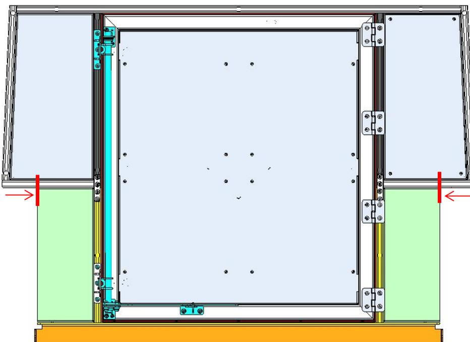
Figure 7: Rear Completed (EPDM Foam Termination Locations)
