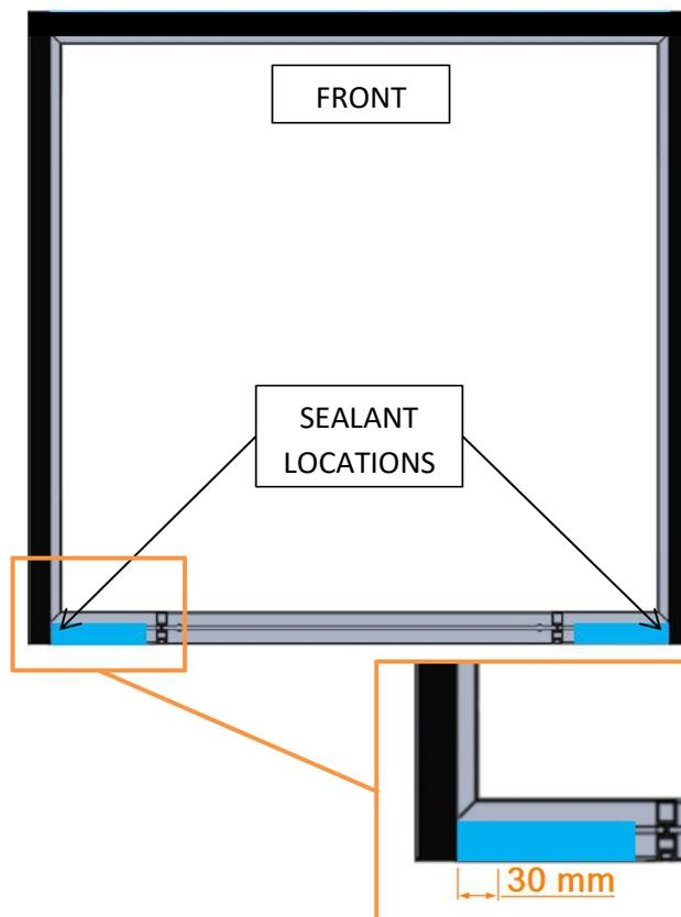
**Figure 6: Rear (Sealant Locations Indicated)**
