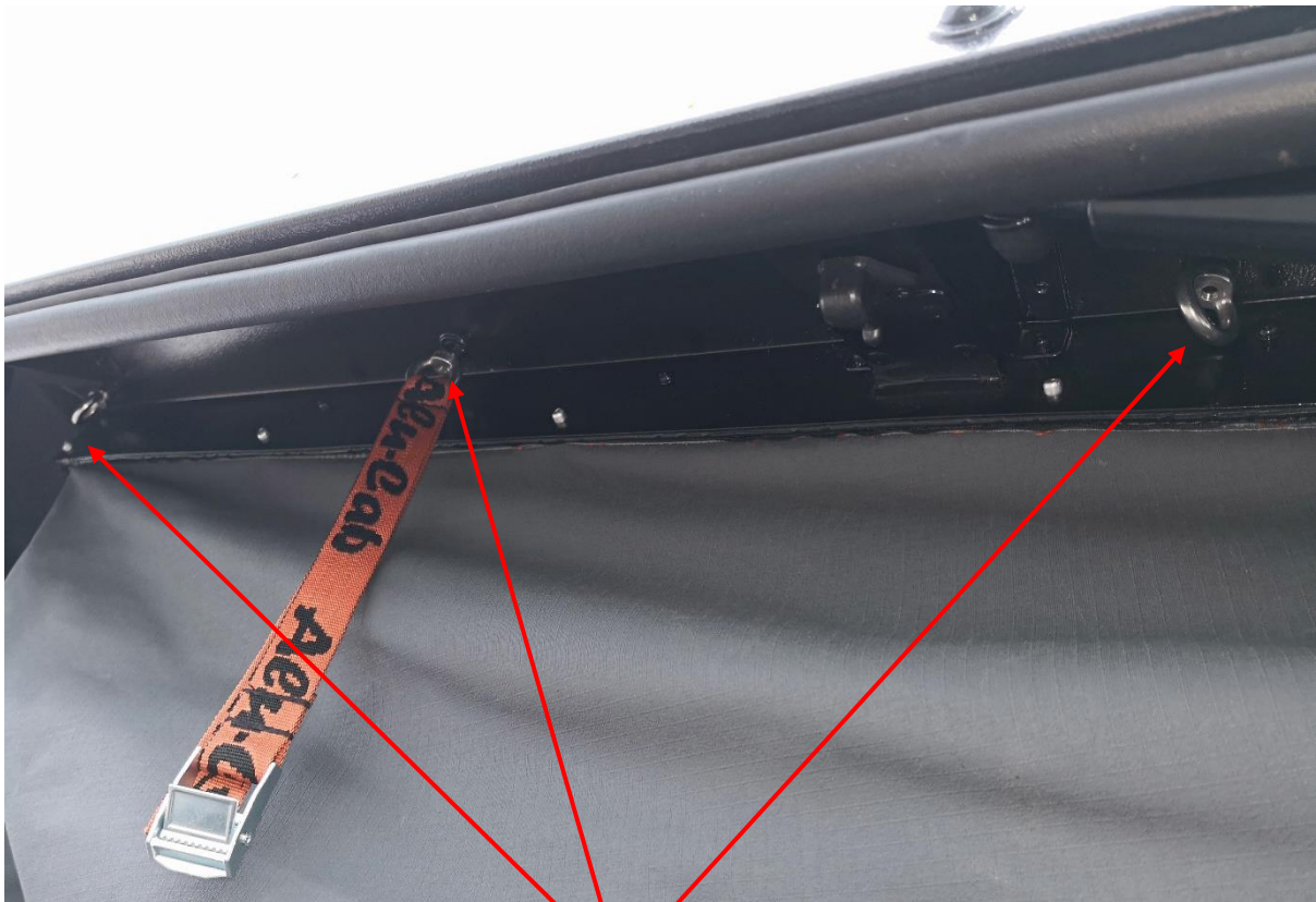
M6 Eye nut & Cam buckle strap with M6 eye nut fastened in the middle.
