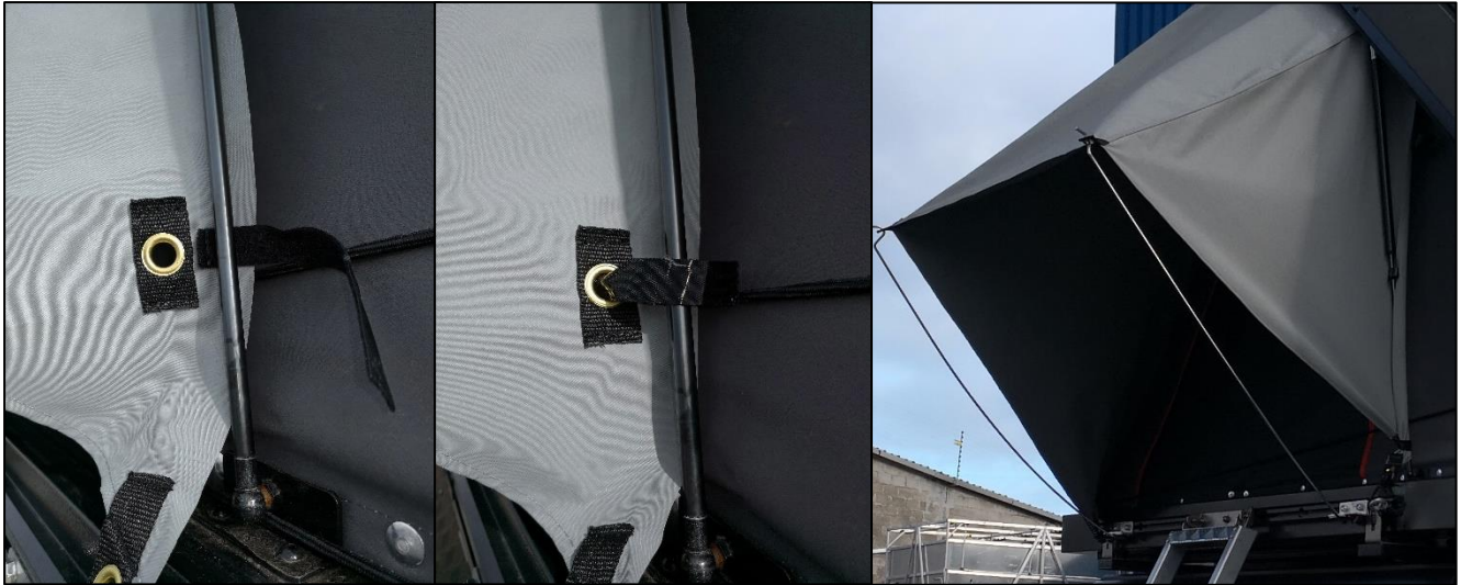
Velcro straps around gas strut to close gap to tent canvas
