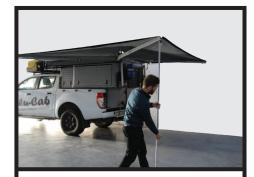
Step 8: With the foot of the centre support leg on the ground, raise the awning slightly, and tighten thumb screw on the pole.
