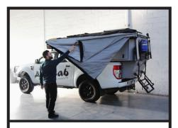
Step 4: Holding the strap, walk around to the front of your vehicle, to the front of the awning frame. Make sure that bystanders keep clear!
