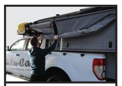
Step 7: When the third canvas fold is exposed, include it into the roll and carry on rolling upwards until the canvas roll is tight against the awning arms.
