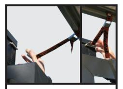
Step 4: Clip the strap onto the rail at the back of your vehicle.
