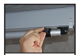
Step 1: If the centre support leg was deployed, loosen its thumb screw and fold the leg up to the awning arm. To secure, slot the support foot into the cradle and then tighten the thumb screw.
