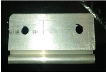
Figure 5: C-Clamp extrusion with holes drilled
