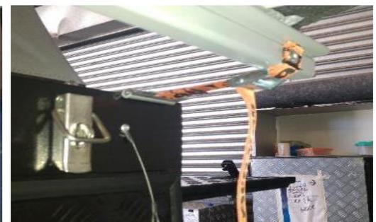
**Step 5:** There are two black adhesive foams strips provided with the awning. Peel the white plastic off and stick these foam strips to the bottom of the awning arms to prevent the side and rear doors of a canopy, camper or any other vehicle from fouling the awning arms.
