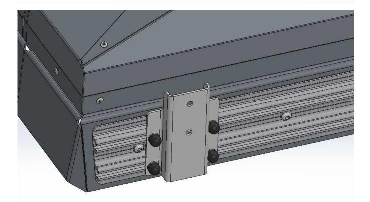
Mount the awning to the brackets, starting from the rear, using the button head bolts and M8 oversized washers.
