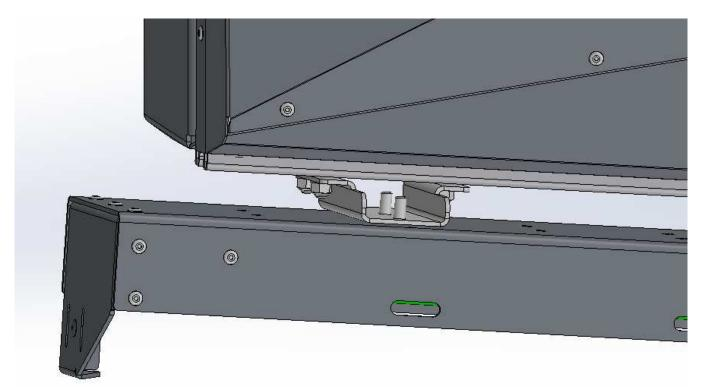
Once the correct positioning for the front bracket is found, remove the awning and tighten the bolts attaching the brackets to the roof conversion and place the black nut-caps on the nuts.
