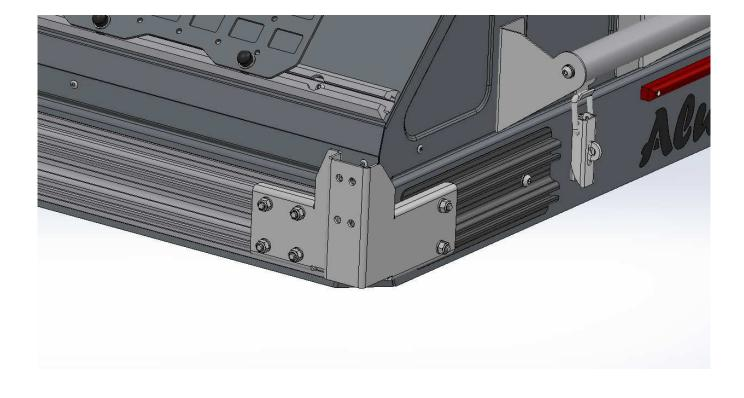
Position the front bracket over the bolts you placed in the front extrusion slots. Fasten the bracket to the extrusion using the supplied nuts and washers.
