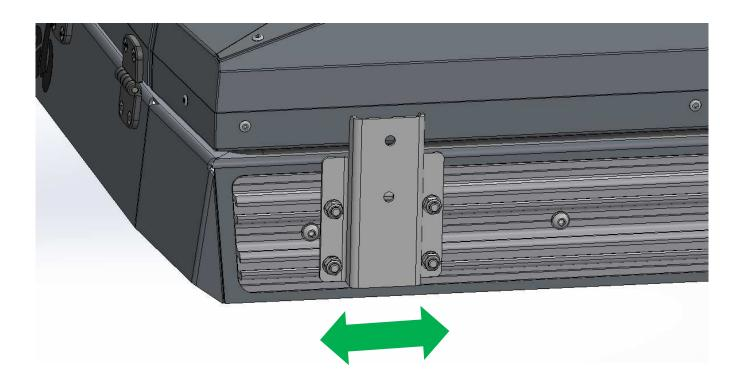
Drill/pierce the awning bag at the 2nd set of mounting holes from both ends (front and rear of the awning).
