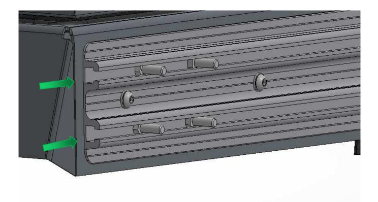
Position the rear bracket over the bolts you placed in the extrusion slots. Fasten the bracket to the extrusion using the supplied nuts and washers.
