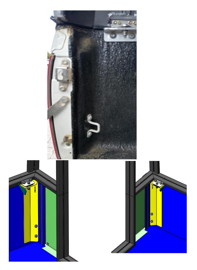
**NB!** The Canopy Camper must rest solely on the mounting brackets and no load is allowed on the load bin. Once this is completed, the Canopy Camper has been installed successfully.
