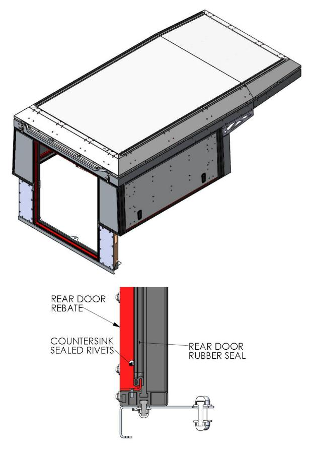
7. Fit rear door by mounting 4 x Butt hinges to camper frame as shown. Centre rear door, top to bottom and the hinge centres left to right. Also mount the door lock to the camper frame.
