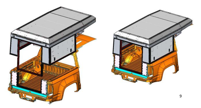
5. Connect rear filler panel assembly and base unit as shown.
