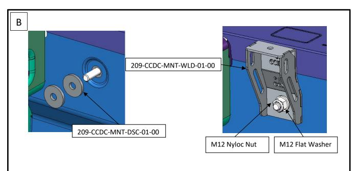
Slide two (2) spacers (209-CCDC-MNT-DSC-01-00) onto the protruding bolt. Then attach the bracket (209-CCDC-WLD-DSC-01-00). Fasten the bracket in place, using an M12 flat washer and M12 Nyloc nut. Ensure that the top surface of the bracket is parallel with the load bin floor.
