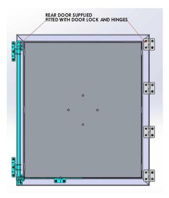
8. Attach hinges and lock to camper frame.
