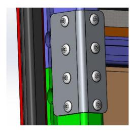
6. Fit rear door rebate with Ø4.8 x15 sealed countersink rivets as shown.
