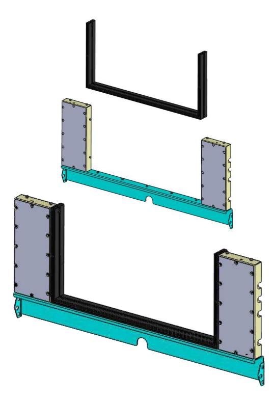
3. Mount filler panel assembly to load bin as shown.
