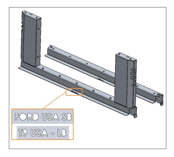
The Rear Filler Assembly is supplied with two (2) different bottom support plates, clearly labeled SB and LB - Ensure that the correct plate is fitted to this assembly, for your specific installation, before progressing.
