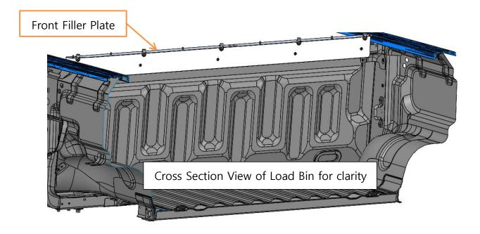
The long lip of the Front Filler Plate mounts up against the front wall of the load bin. A generous amount of sealant should be applied in an unbroken line, encircling the holes, on the interface surface. The plate will be drilled and riveted to the load bin, in position.
