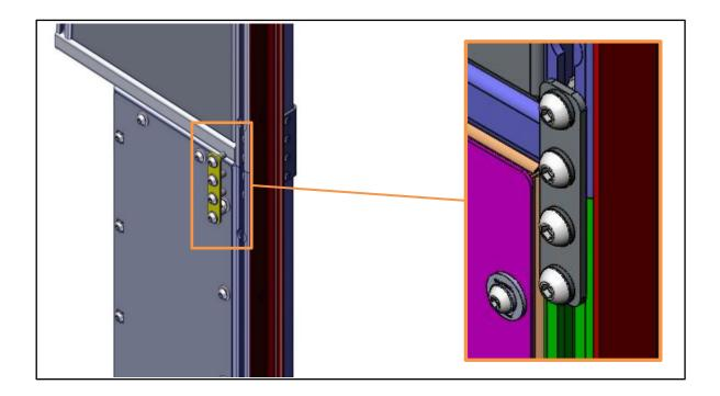
Using the supplied hardware, fasten the lower and upper door frames together, on each side of the **INTERNAL** door opening. See images below:
