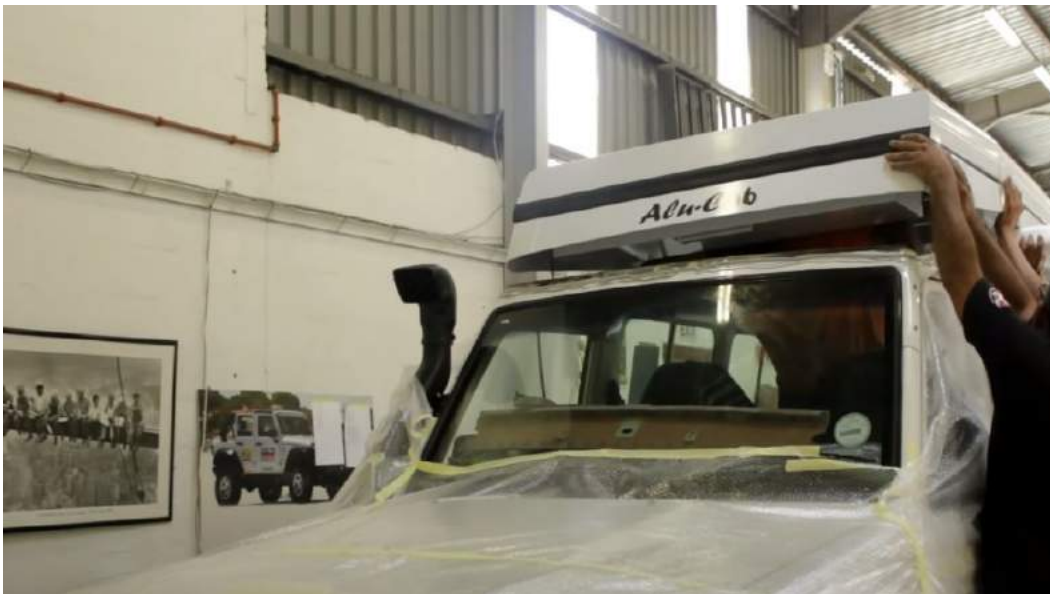
Clamp down the roof on the rear and sides of the vehicle for a proper seal.
