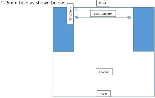
The measurements might vary depending on your load bin, but try to stay within the sizes indicated in the above diagram. Fasten the chain assembly as shown below:
