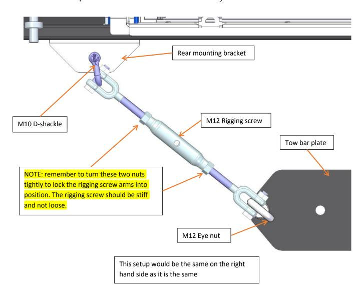
NB: In some cases there may be a metal chain in the rigging screw assembly to accommodate for Length variants.
