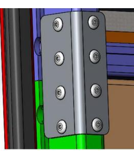
Fit rear door rebate with Ø4.8 x15 sealed countersink rivets as
