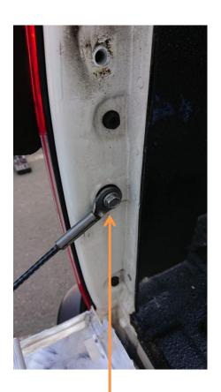
Do not discard this fastener, it is reused to mount the filler kit
