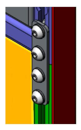
**INNER MOUNTING ON BOTH JOINTS**
