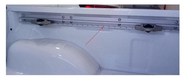
2.1 Fit 3 off mounting bracket set on either side of load bin to the pre fitted rail as shown above. Insert nut plate of bracket set into rail and bolt the bracket onto it.
