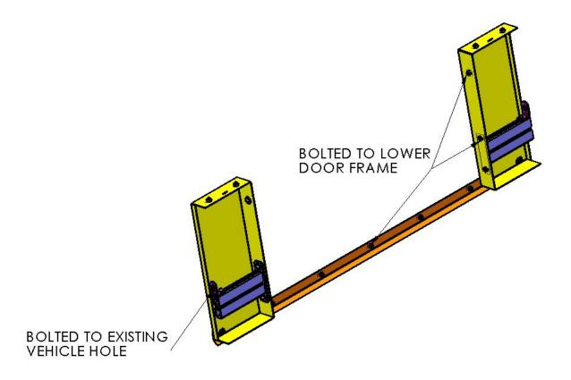
Fit lower door frame to filler panel assembly as shown.
