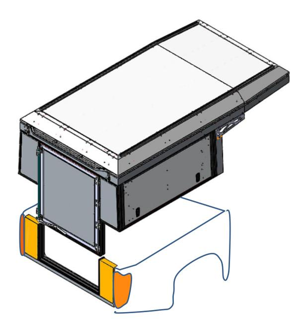
1. Connect rear filler panel assembly and base unit as shown.
