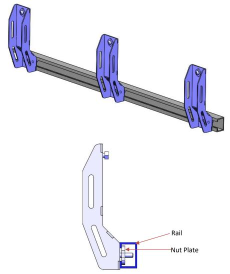
3. Fit top bolt of bracket into base frame load bar as shown below.
