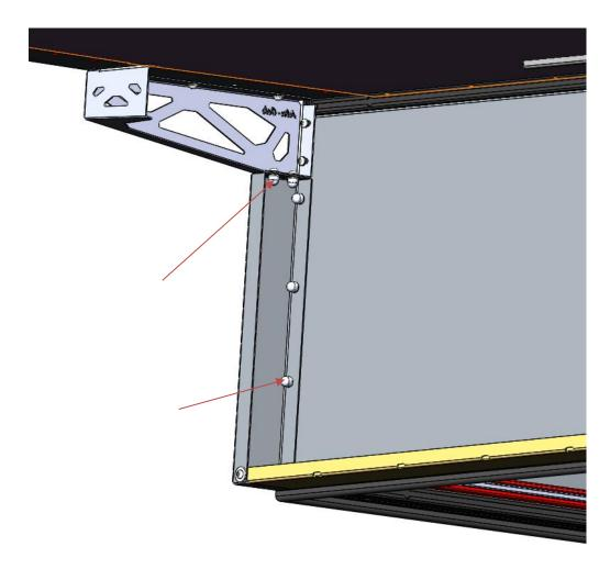
Rivet bottom filler panel on to bottom frame member using supplied Ø4.8x15 sealed rivets
