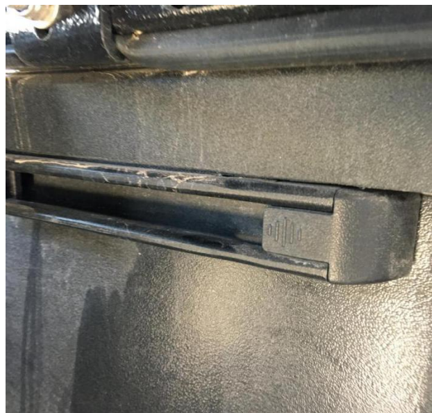
Figure 1: The above Plate with threaded holes is inserted into the below rail inside the Load Bin
