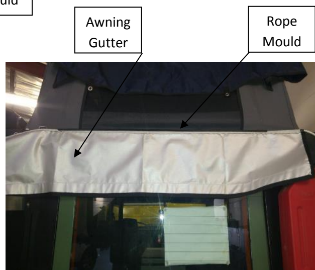
Figure 12: Gutter Installed into Rope Mould
