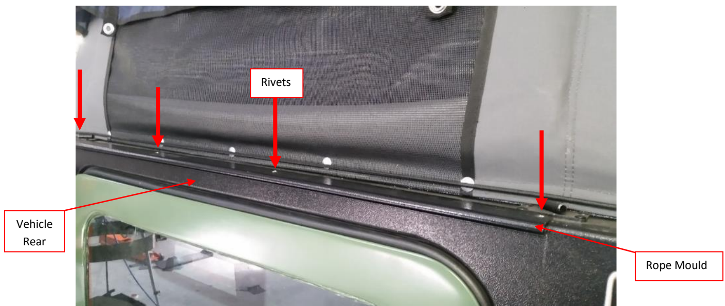
Figure 8: Rope Mould mounted onto Vehicle
