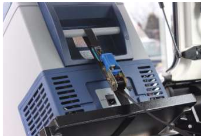
Figure 6: Ratchet strapped fridge.
