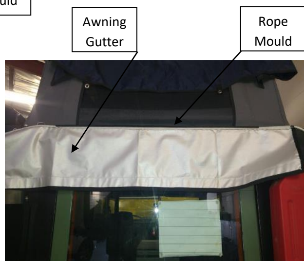
Figure 12: Gutter Installed into Rope Mould
