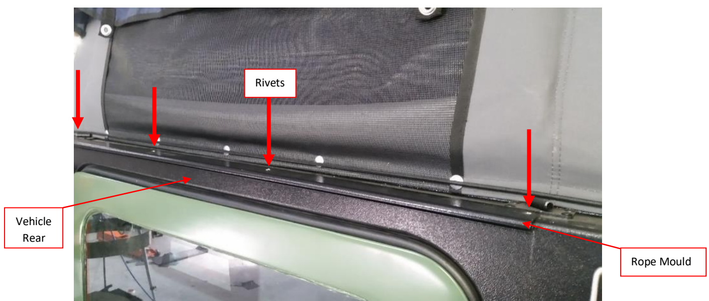
Figure 8: Rope Mould mounted onto Vehicle
