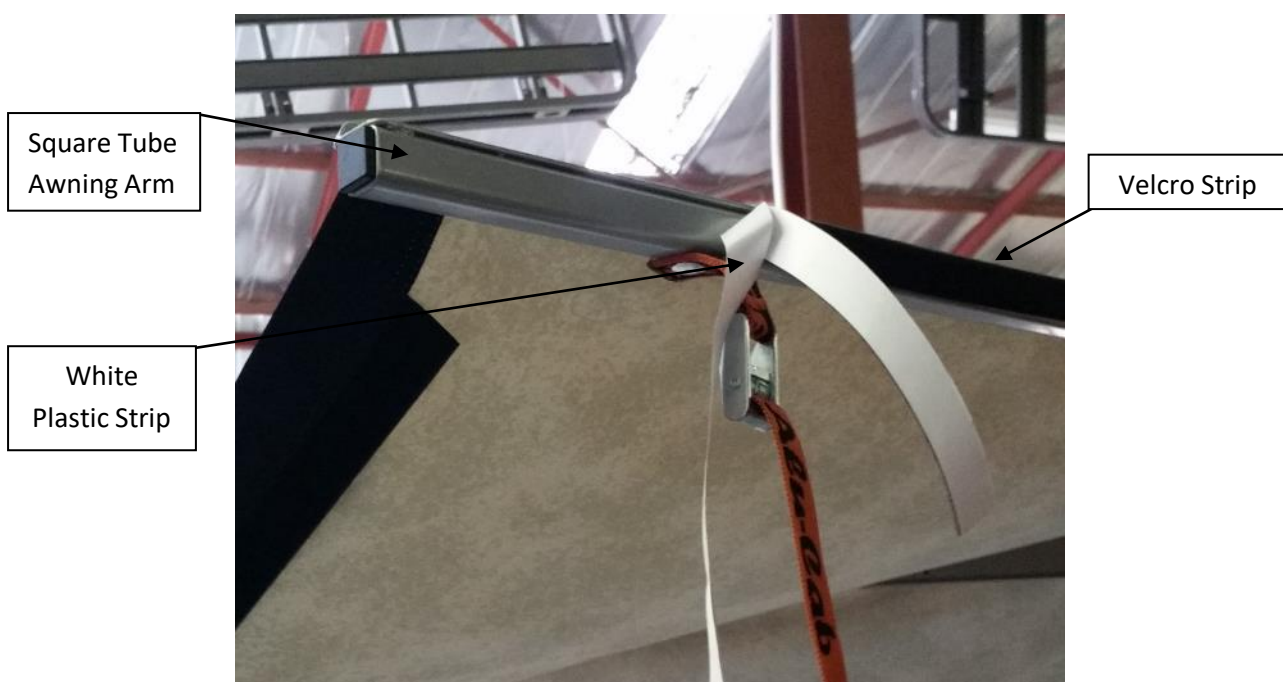
Figure 9: Removing White Plastic Strip
