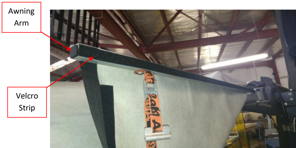
Figure 10: Velcro Strip Fitted to Awning Arm
