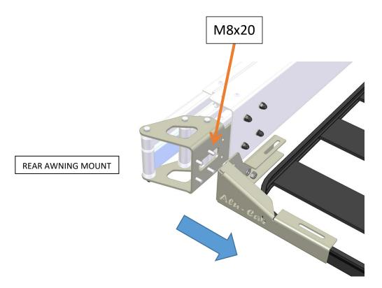
Line up the supplied brackets and and the awning to check that the awning's 270deg arm clears the vehicle.
