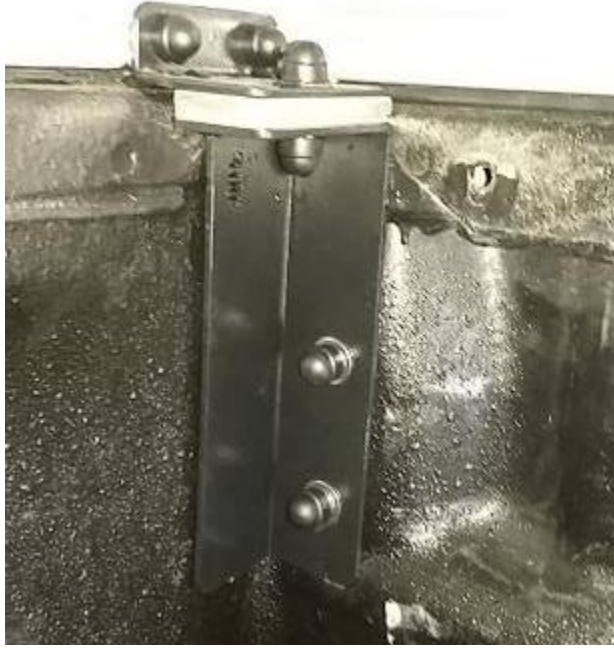
Figure 16: Front Support Bracket Installed
