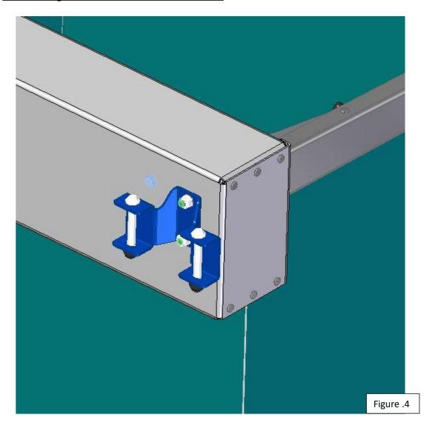
Remove the two M8 Nyloc nuts from the shower cube and fit the bracket (492-FRUN-FNT-MNT-BRKT-01) to the shower cube.
