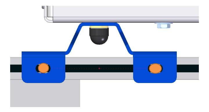
Use the slots on the brackets as a jig to drill 8.5mm holes to fit the M8x70mm bolts.
