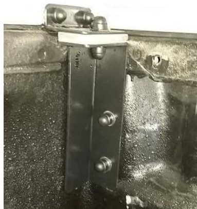
Figure 20: Mounting Universal-Front Support Bracket
