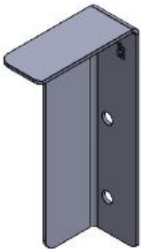
Figure 4: Isuzu Canopy Mount – IRF (Right Front)
