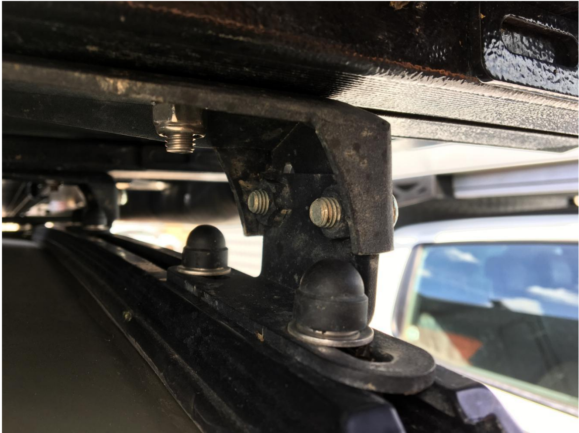
Figure 4: K9 Mounting Bracket on Front Runner Roof Rails
