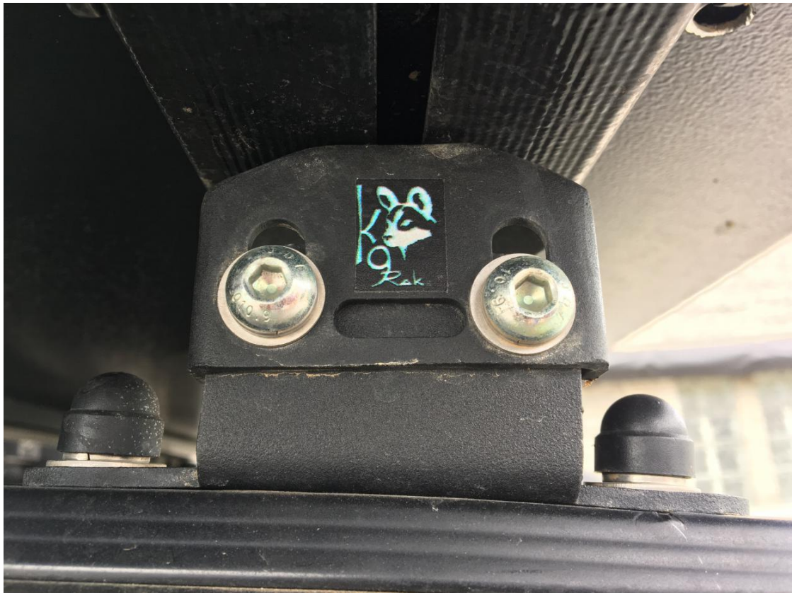
Figure 10: Button Head Allen Key Bolts For Adjustment
