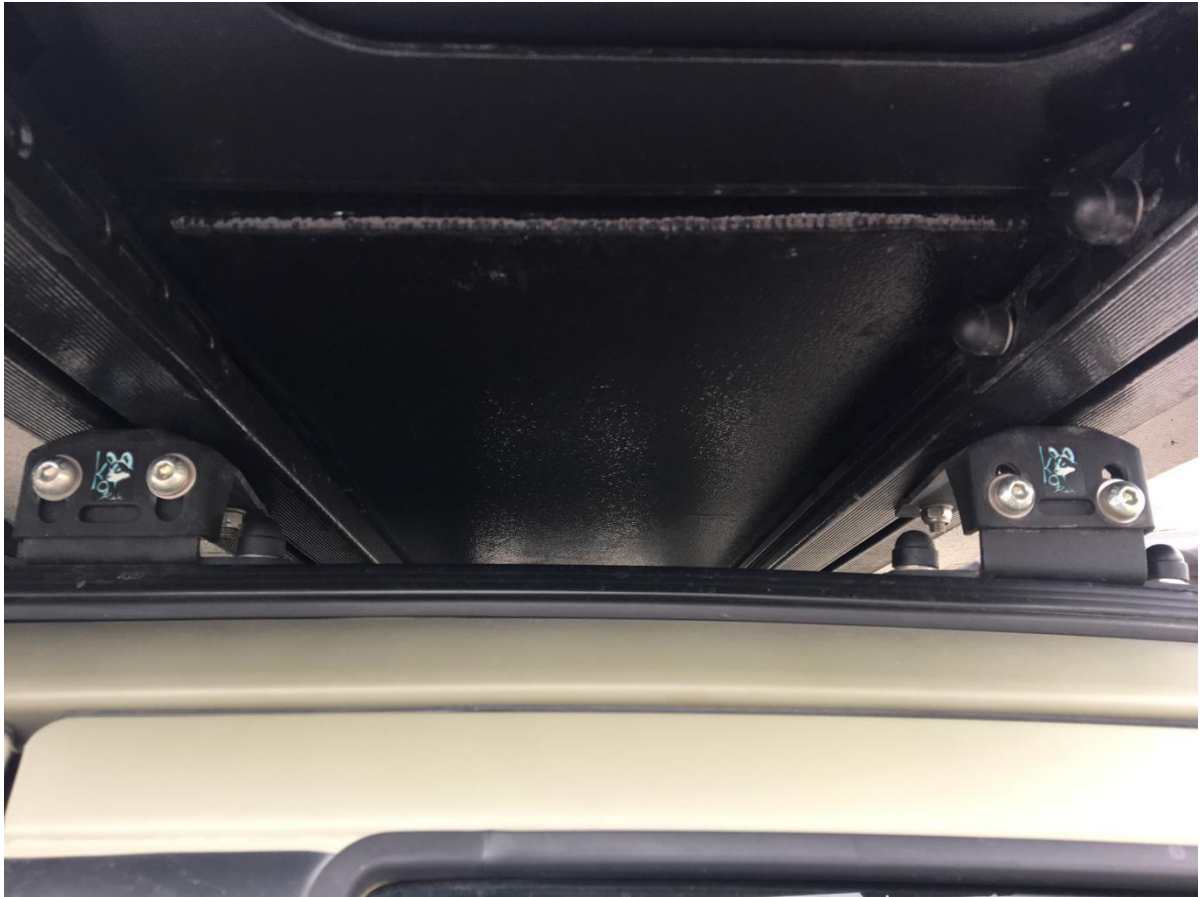
Figure 12: K9 Mounting Brackets and Load Bars Leveled
