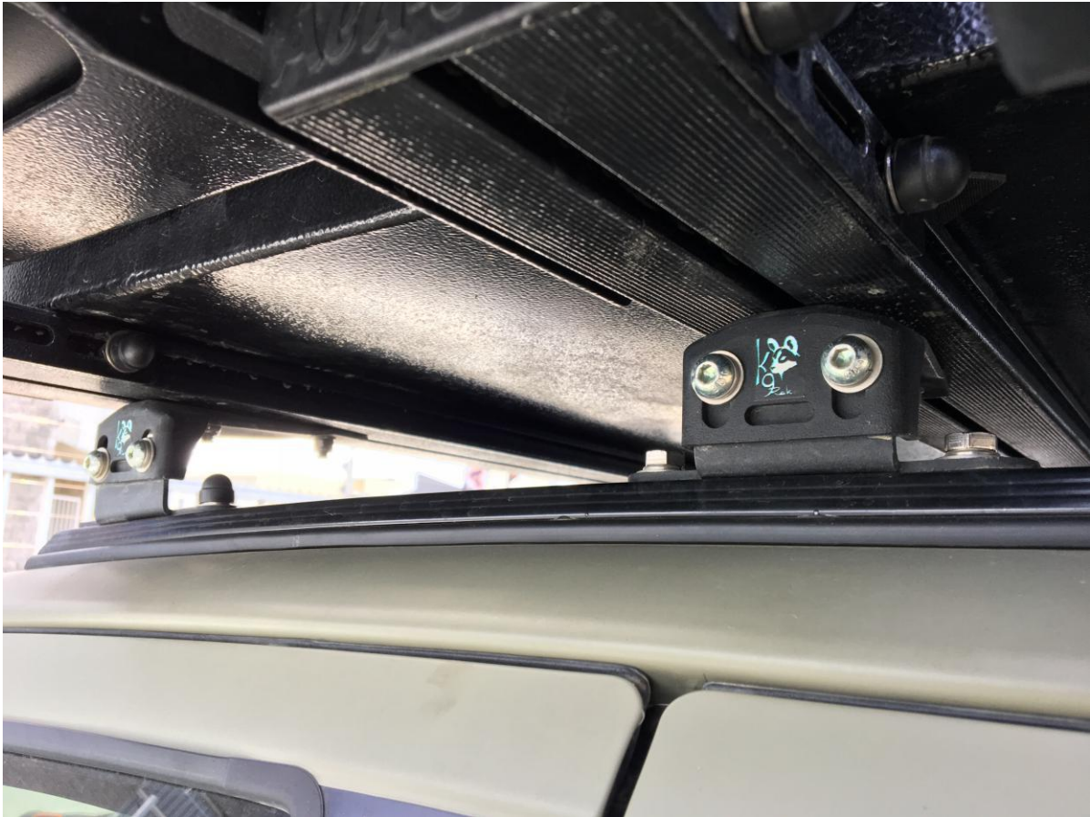
Figure 6: K9 Mounting Bracket on Front Runner Roof Rails
