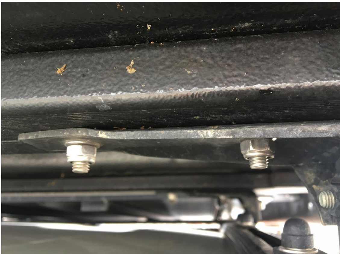
Figure 8: Hex Bolts Located and Fastened to Horizontal K9 Bracket Component
