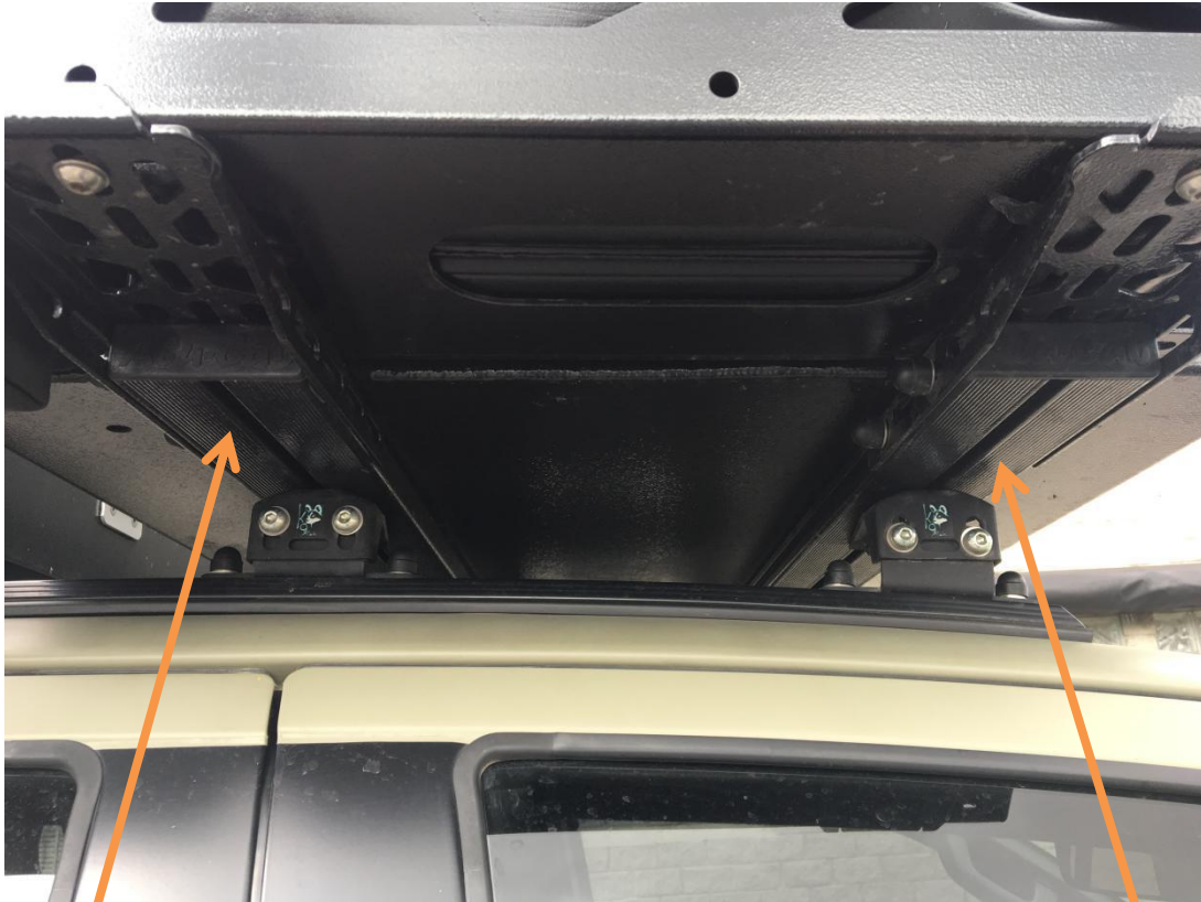
Figure 9: Making the Load Bars Parallel and equidistant
