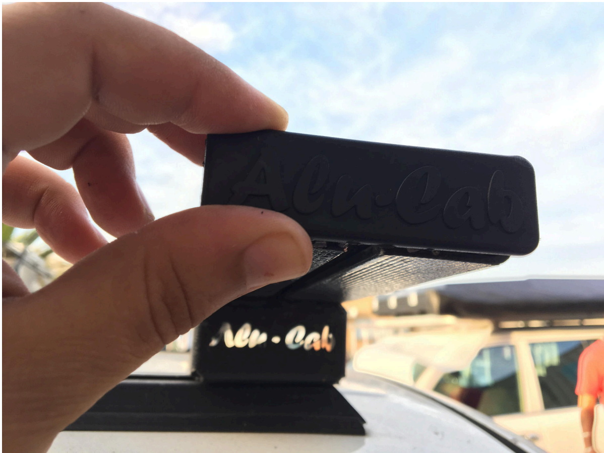
Figure 4: You may need a tool to pry it off of the Load Bar
