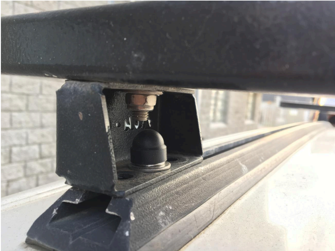
Figure 7: Fastened Load Bar to Mounting Bracket
