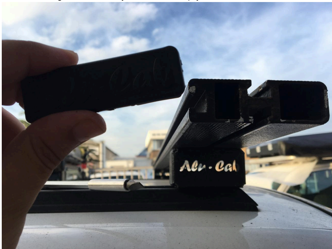
Figure 5: Remove the End Cap once loose
