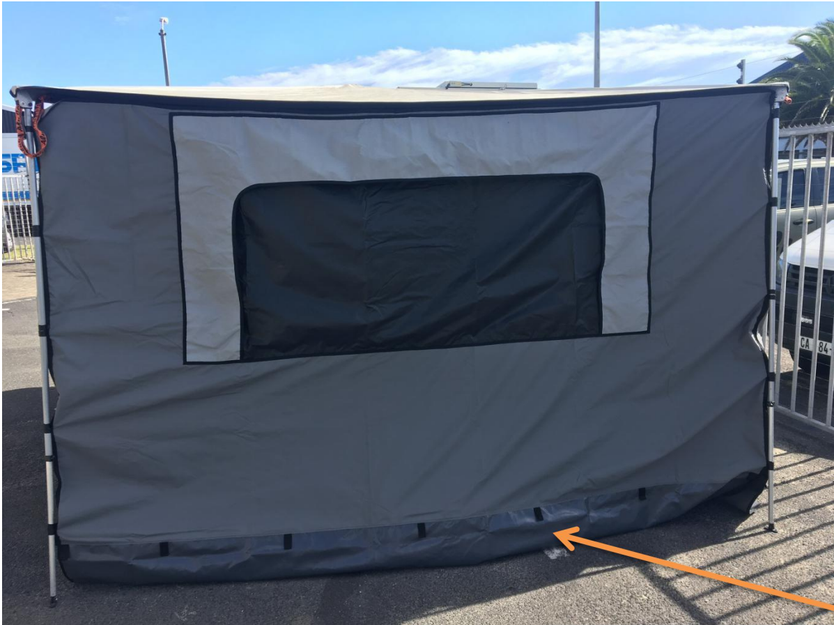
Figure 20: The Number 2 Side Canvas attached with the Zip, Top Velcro and Side Velcro Straps. *Note the Lower Loops for your Tent Pegs to go through
