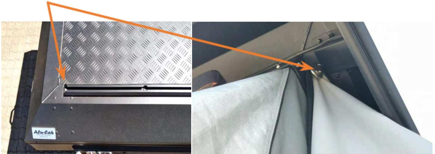
**Bolt 2:** (the sixth bolt from the front end of the cargo rail, situated inside the lid of the tent)
