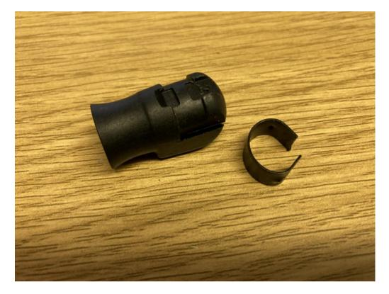
Now the gas strut ends can be transferred from the old struts to the new struts by unscrewing them off of the old and screwing them onto the new.
