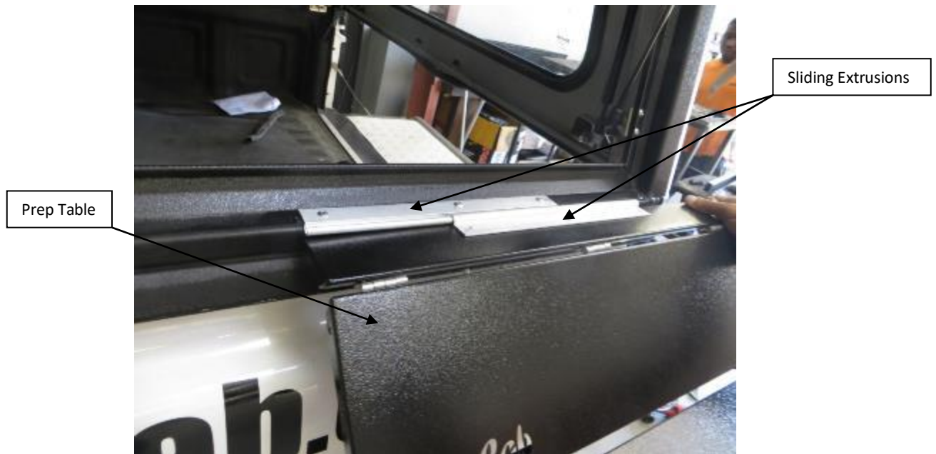
Figure 8: Sliding Prep Table into Rope Mould
