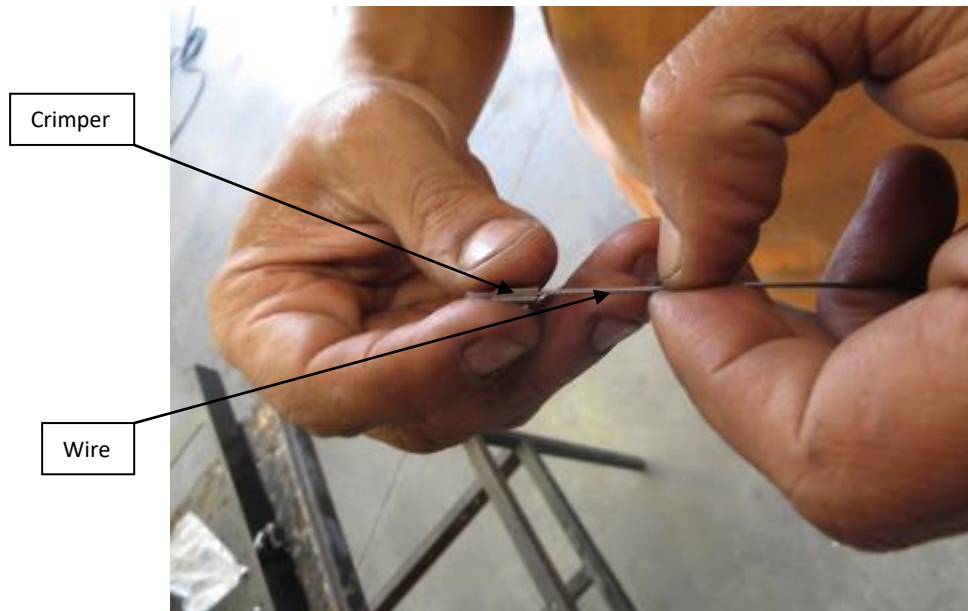
Figure 10: Inserting wire into 1 side of crimper
