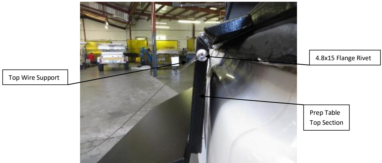
Figure 14: Rivet Top Wire Support
