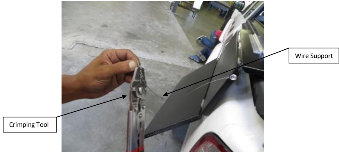
Figure 16: Crimping other end of wire support
