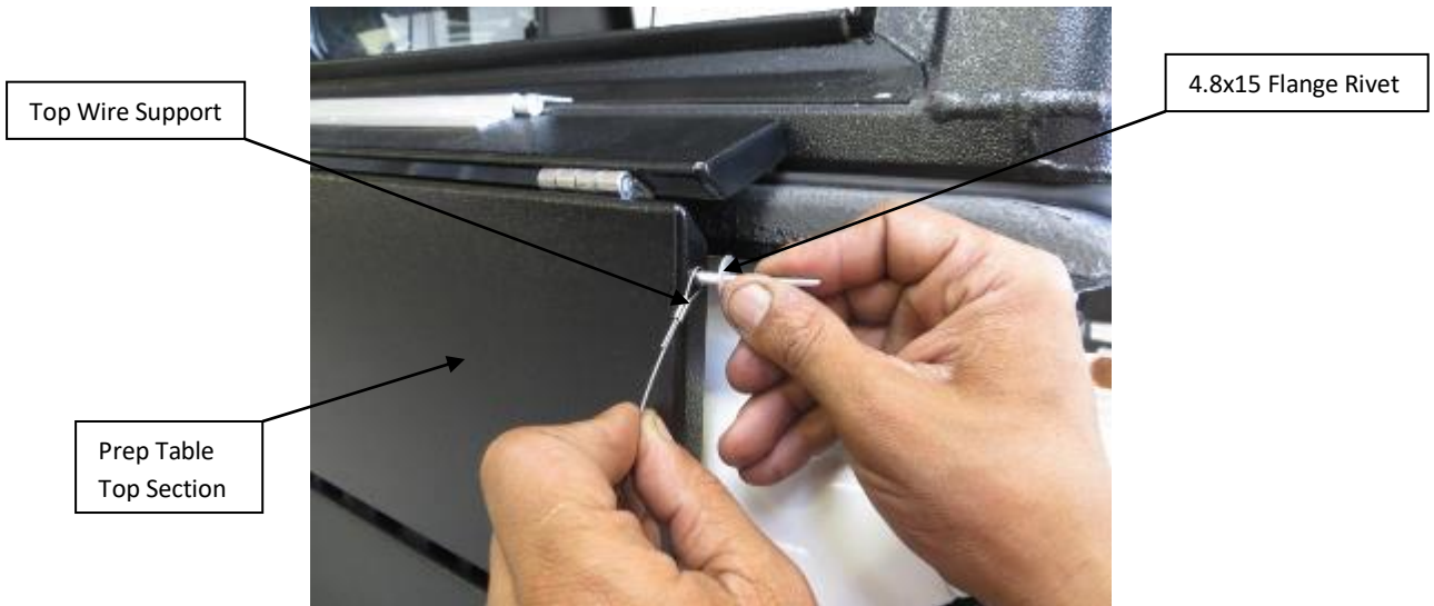
Figure 12: Adjusting Crimper for a close fit
