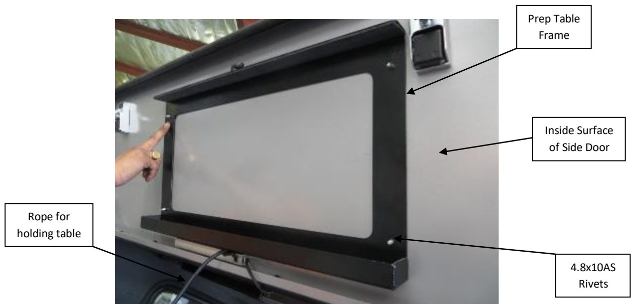
Figure 24: Prep Table Frame installed
