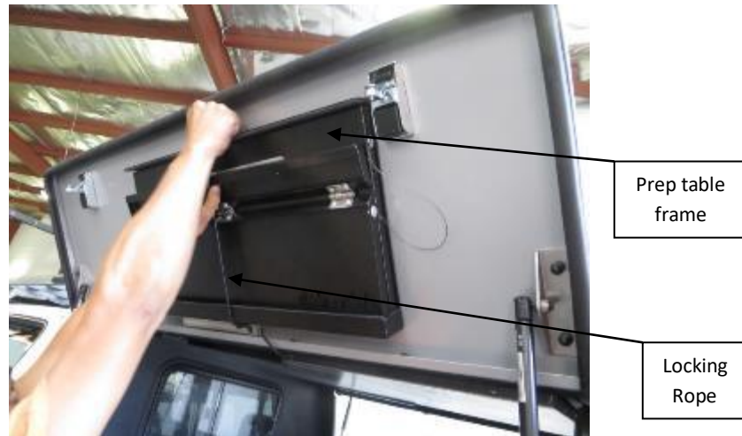
Figure 26: Fixing table in place
