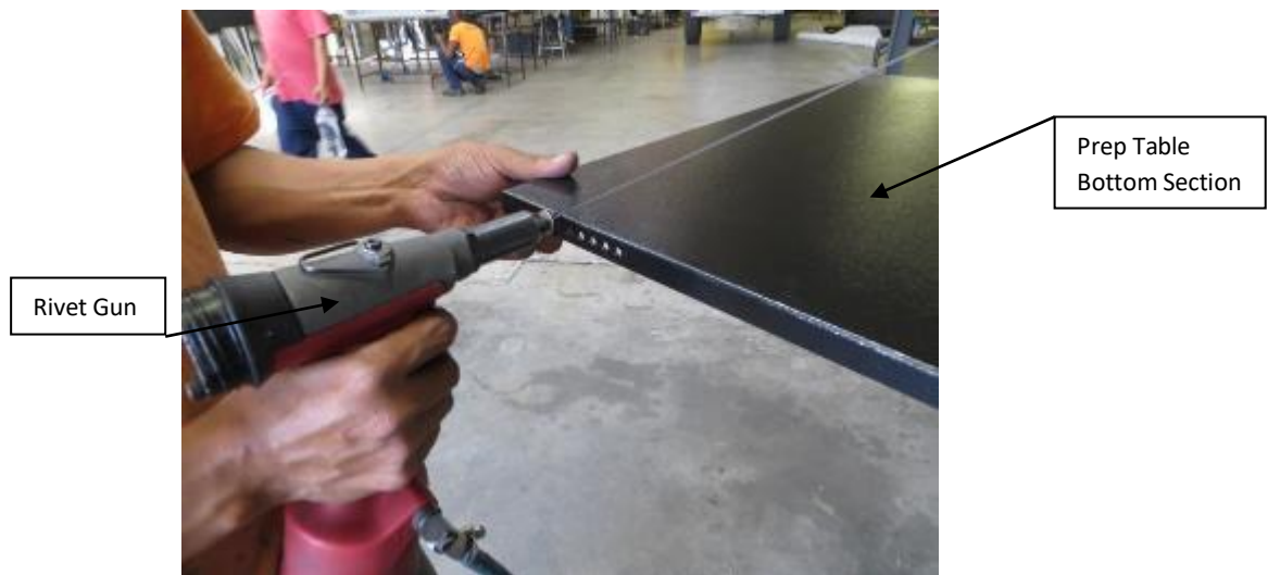
Figure 17: Rivet bottom wire support
