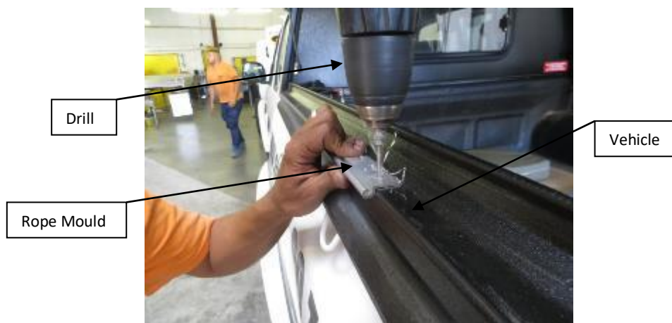
Figure 5: Drilling Mounting Holes into vehicle
