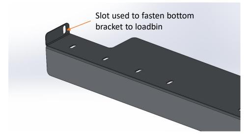
With the bottom bracket installed, the next step in the process is to mount the lower door frame of the canopy camper to the bottom bracket. This is done by sliding five M8x20 hex head bolts (item 7) into the bottom frame and lining them up with the slots in the bottom support bracket. Push the bolts through the slots and fasten them loosely using a M8 Nylock nut (item 6) and washer (item 8).
