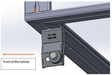
The rear brackets use a top mount bracket (209-CCDC-TOP-BRK-01) to fasten to the Canopy Camper Frame.
