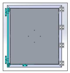
Insert the assembled door into the rear door opening. Fasten the four (4) hinges into the nut slot on the RHS door frame first, using the supplied hardware.
