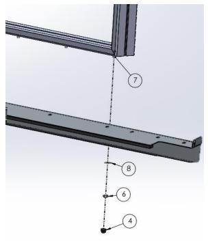
With the bottom door frame installed the last part of the installation for the rear filler kit is adding the side filler boxes.
