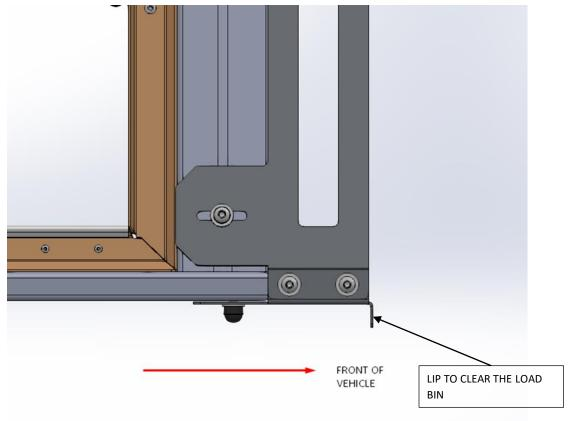
The last step is to seal the front filler with Black UV Sikaflex as indicated below
