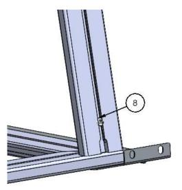
Next fasten the left and right brackets to the bottom filler bracket, and then to the Canopy Camper frame itself
