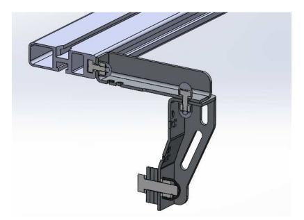
Once all the brackets are in their correct positions they can be fastened down securely using a 13mm socket for the M8 nut and bolts and a 18 mm socket for the M12 bolts and nuts. A ratchet will also be required.
