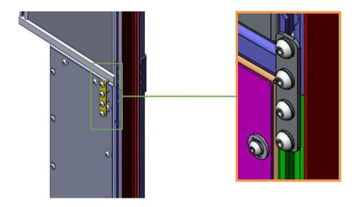
Using the supplied hardware, fasten the lower and upper door frames together, on each side of the **INTERNAL** door opening. See images below:
