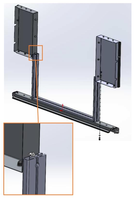
With the side filler boxes in position fasten them down to the bottom filler bracket using the supplied hardware. The setup is like fitting the bottom door frame, there is just an addition of a flat washer on the inside of the box, and some plastic nut caps to finish the look off.
