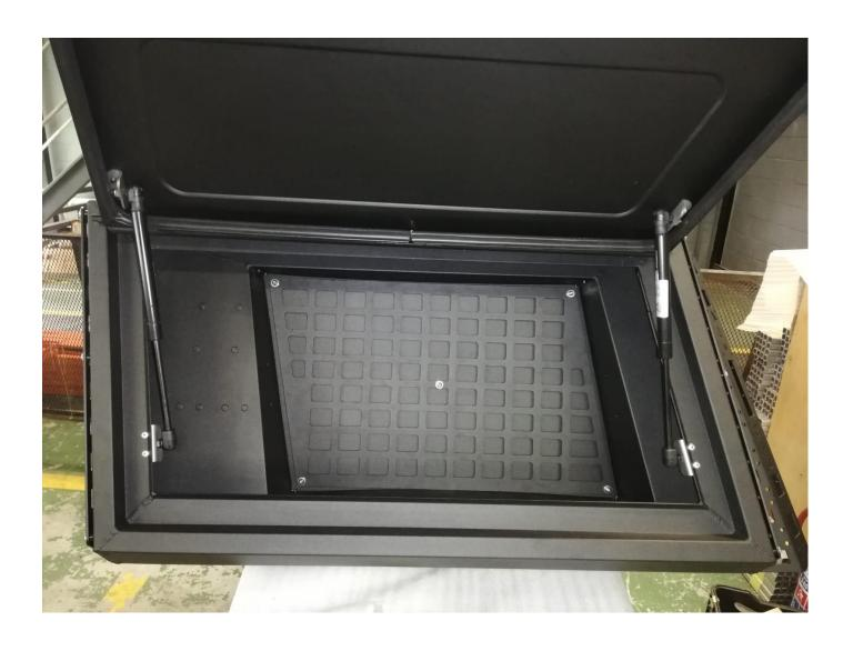
Once the backing plate is securely bolted down, and the rubber matting is in place, you will have successfully installed the recovery molle plate kit to your window box.
