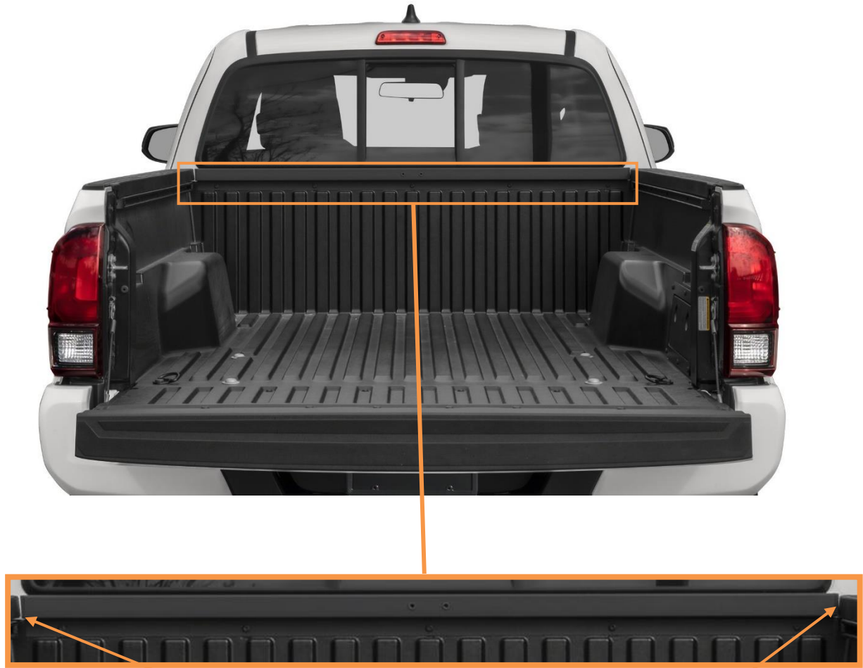
Fig 12: Gaps in Factory Bulkhead Spacer
