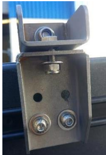
Fig 11: Photos of Bracket kit assembled in Tacoma Load Bin
