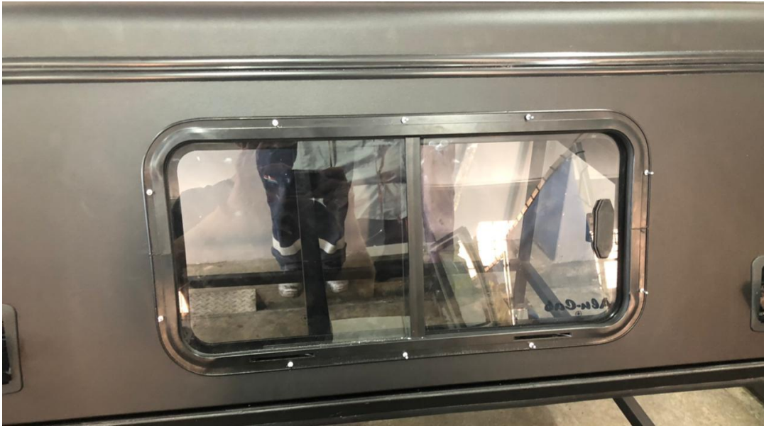
Figure 7: Inserting window into canopy and rivets into drilled holes.
