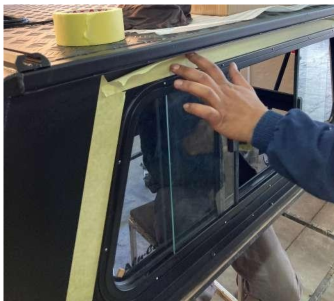
Figure 10: Cover canopy around sliding window with masking tape.
