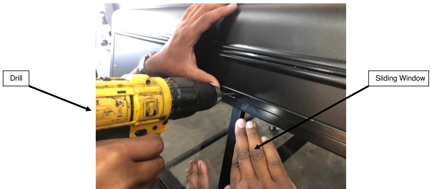
Figure 4: Drilling the holes to place rivets
