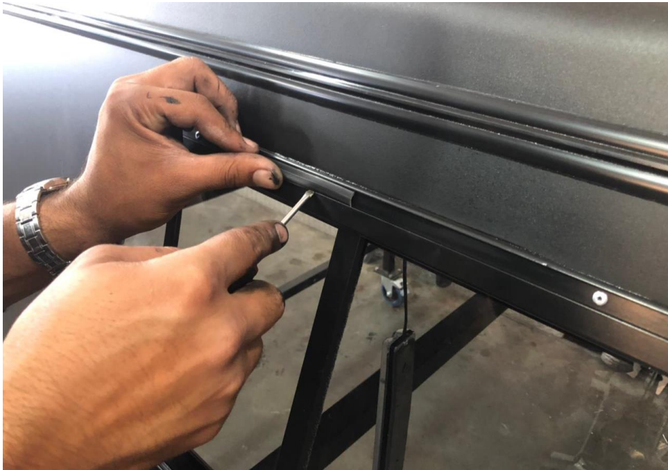
Figure 11: Adding new rubber to sliding window.
