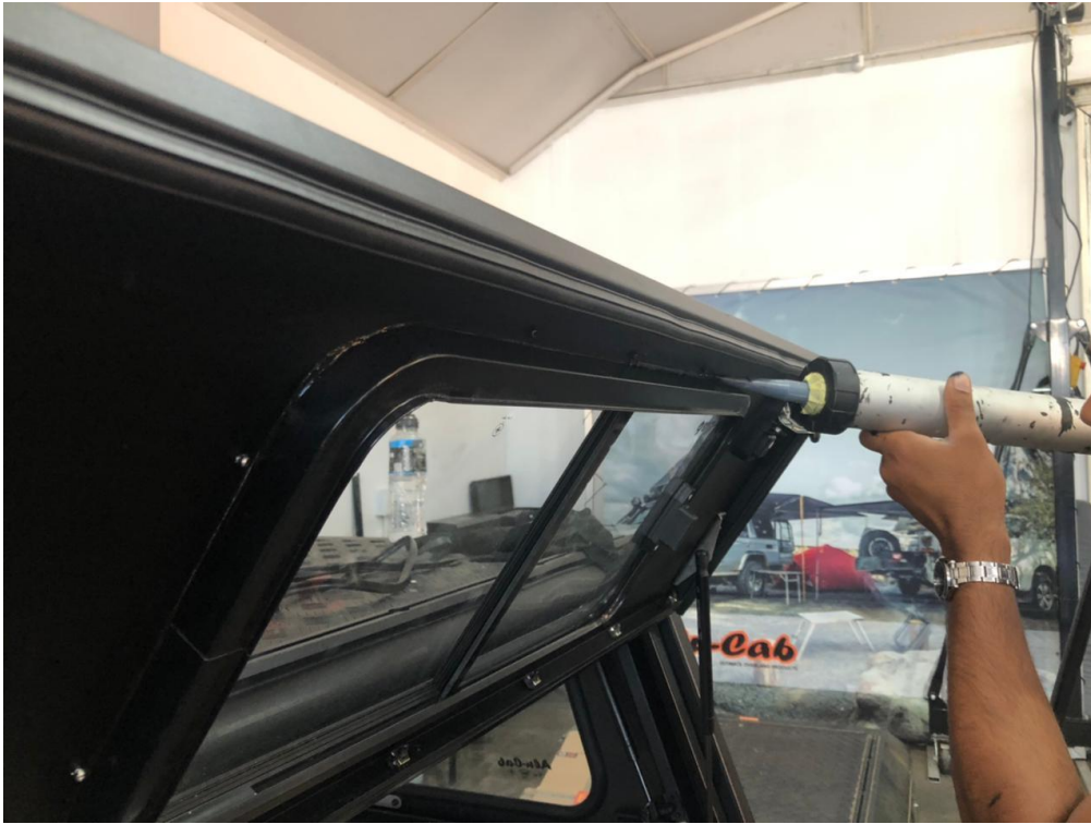
Figure 9: Add sealant on inside of window.
