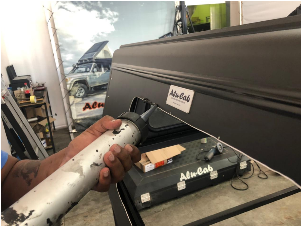
Figure 6: Add Sikaflex/Sealant to outside of window.
