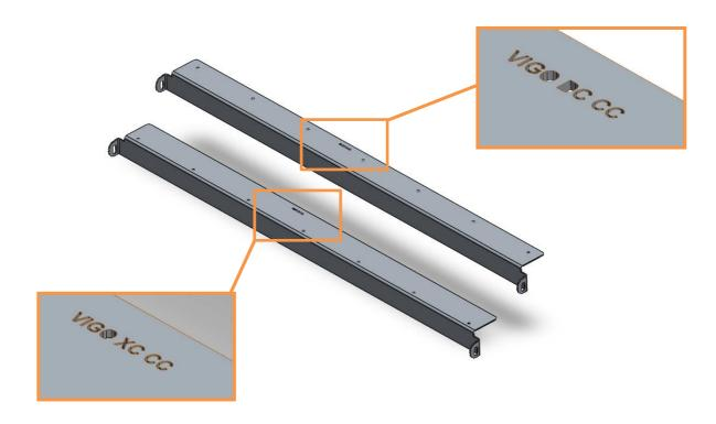
Choose the correct brackets to be used in the correct application. The bottom support bracket annotated as *VIGO XC CC* should be used on the Extracab (XC) variety of the Hilux Vigo. The bottom support bracket annotated as *VIGO DC CC* should be used on the Doublecab (DC) variety of the Hilux Vigo.
