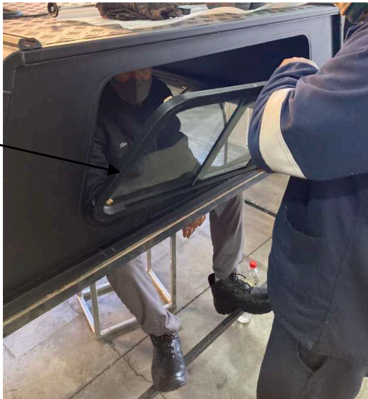
Figure 6: Placing sliding window for drilling
