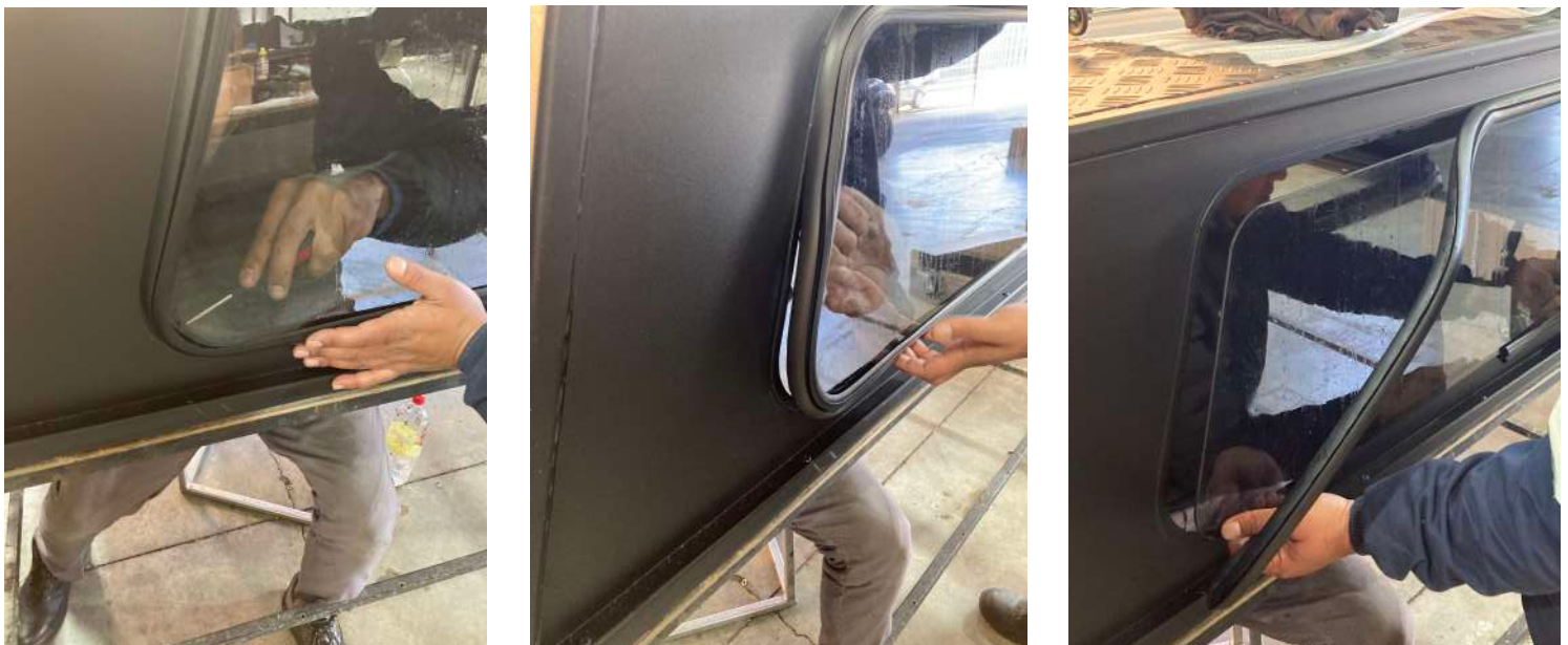
Figure 3, 4 & 5: Removing rubber + window
