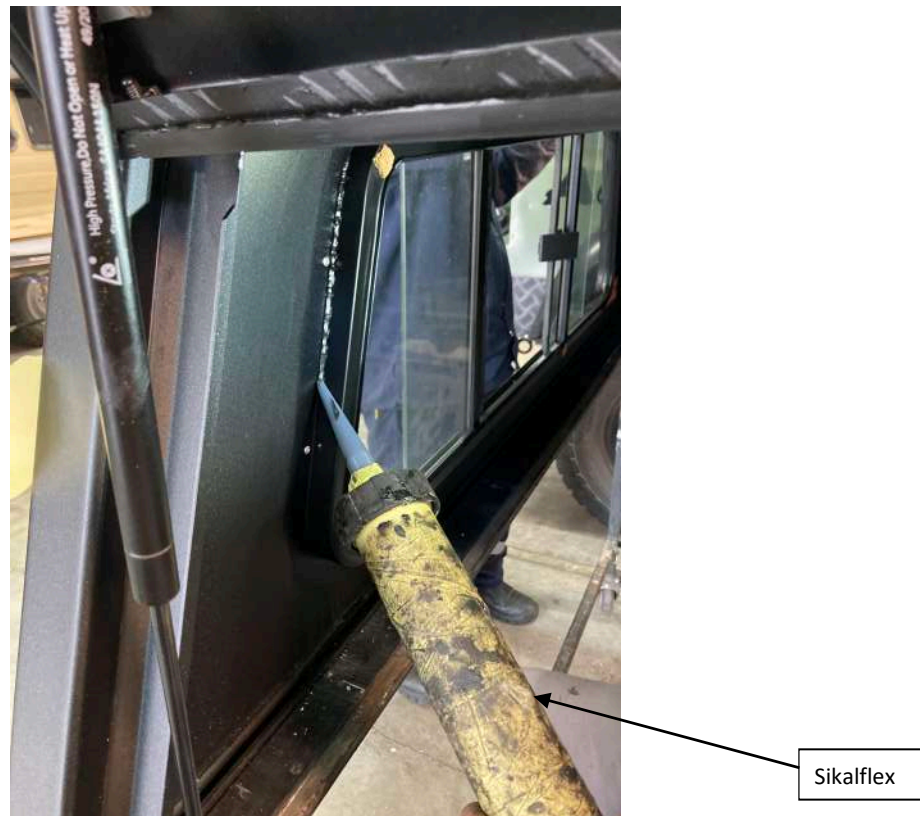
Figure 12: Add sealant on inside of window.
