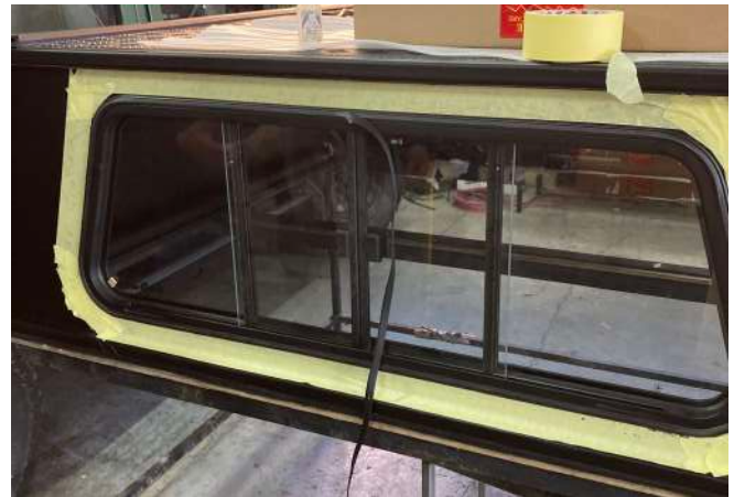
Figure 14 & 15: Adding new rubber to sliding window.
