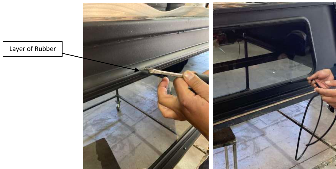
Figure 1: Cutting into rubber.
