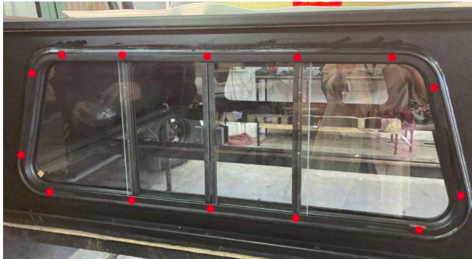
Figure 8: Where holes need to be drilled.
