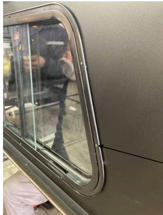
Figure 10: Inserting window into canopy and rivets into drilled holes.
