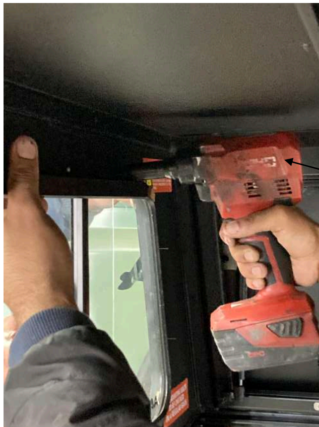
Figure 11: Use rivet gun to fix rivets to window.
