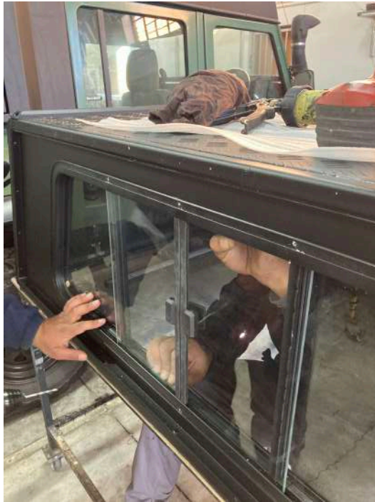
Figure 10: Inserting window into canopy and rivets into drilled holes.
