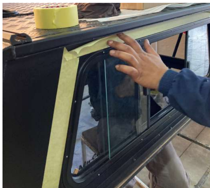
Figure 13: Cover canopy around sliding window with masking tape.
