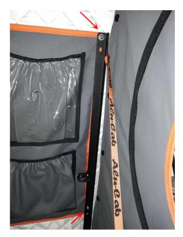
NB: If you have a Gen3 or 3.1 tent you will have rivets instead of riv-nuts. So we have supplied 4 off 4.8x21mm large flange rivets so you can drill the corner rivets out and pop the brackets into place. If you have bolts and the thread is spoilt, then you can use the rivets to replace the bolts as well.
