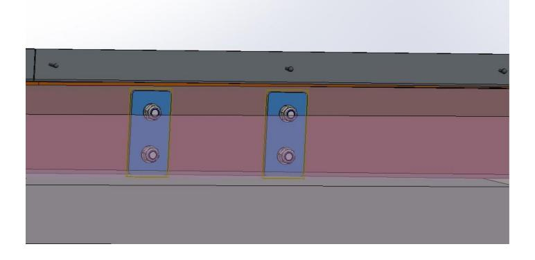
After tightening up the fasteners, wipe away any excess sealant that has squeezed out past the brackets, on the outside surfaces. The preferred cleaning agent is a 50-50 mixture of isopropyl alcohol and water. Refrain from using harsh chemicals, as they may damage the powder coating.
