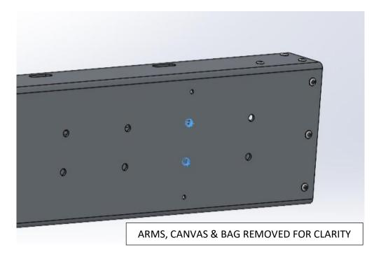
At the rear of the Shadow Awning, at the pivot point plate, count the hole pairs from the rear, and drill through the bag at hole pair one (1), as shown in the image below. Ensure that the arms, and/or canvas is safely out of the way before drilling. Use an  $\Phi$ 8.5 mm drill bit.
