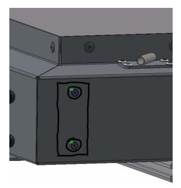
Fasten the rear bracket using the bolts, washers and nuts supplied. Ensure the tent panel is sandwiched between the rear bracket and the accompanying backing plates as in the images below:
