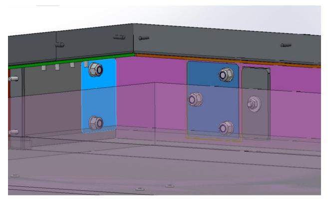
After tightening up the fasteners, wipe away any excess sealant that has squeezed out past the brackets, on the outside surfaces. The preferred cleaning agent is a 50-50 mixture of isopropyl alcohol and water. Refrain from using harsh chemicals, as they may damage the powder coating.
