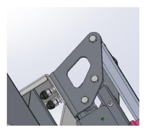
Align the front of the Shadow Awning, with the installed front bracket, as shown below. Insert the fasteners, as per the section *Component Identification*. Ensure that the awning is seated correctly, and not leaning forwards or backwards. Tighten these fasteners, and then tighten the fasteners on the rear corner bracket.
