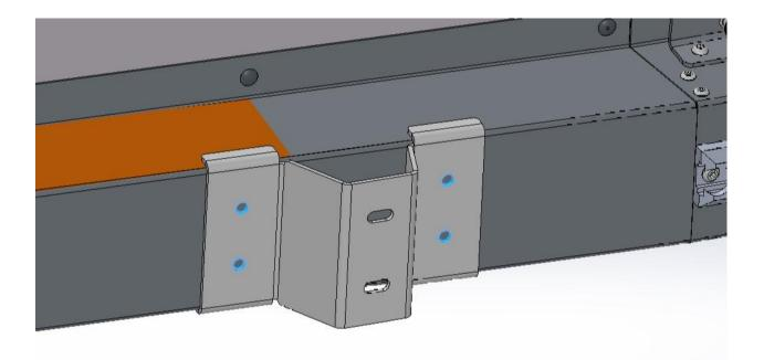
Apply unbroken beads of sealant around all the drilled holes, as well as making an unbroken bead around the perimeter, within the bounds of where the bracket will mount. Use the same technique, as described in *Fitment of Rear Mounting Bracket*.
