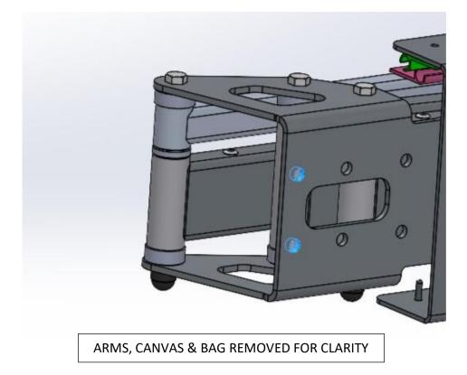
Align the rear of the Shadow Awning, with the installed rear corner bracket. Insert the fasteners, as per the section *Component Identification*, do not fully tighten the fasteners.
