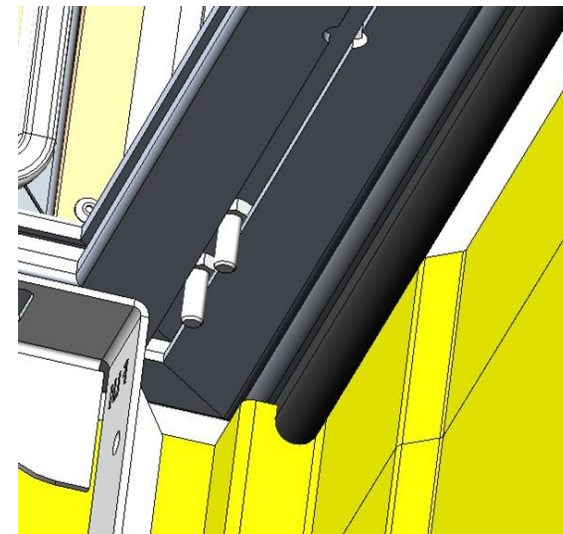
Figure 8: Slide 2x M8x20 hex bolts into nut slot on the camper frame
